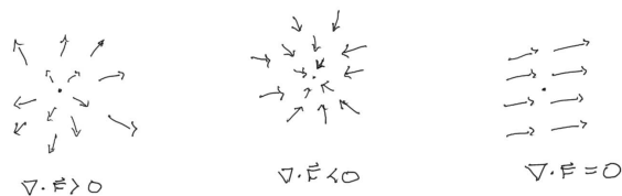
Figure 6.14: A source of a vector field is a point with positive divergence while a sink is a point with negative divergence.
