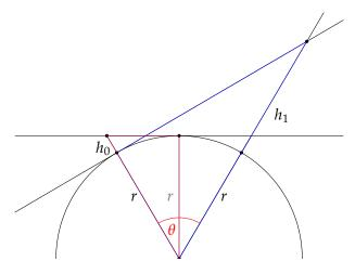
Initially, the two astronomers are each a height of  $h_0$  above the ground at their towers. For the two astronomers to just barely see each other, the line segment connecting them must lie tangent to the planet at the midpoint between them. Taking the important bits of the geometry from this setup gives us the following right triangle.
